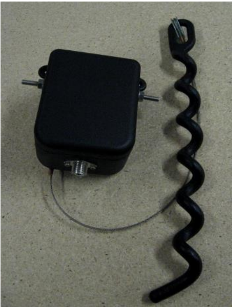
Above: Bushcomm Balun showing pigtail strain relief feature***
