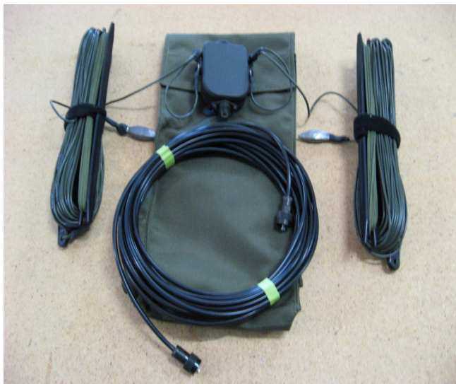
Tactical Tuned Dipole unpacked with Coax Cable
