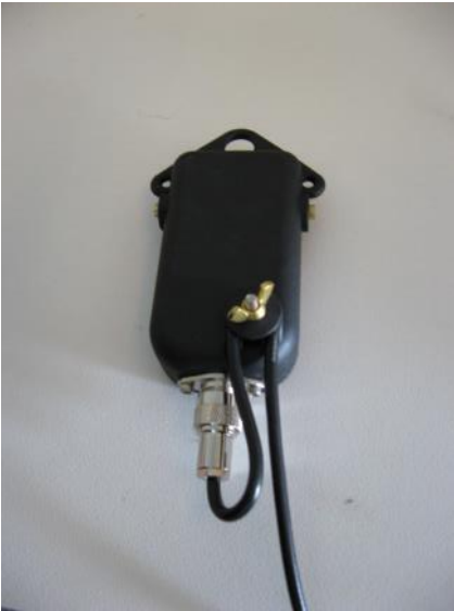
Above: Bushcomm Balun showing coaxial strain relief feature***
